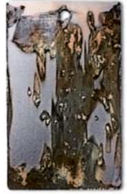
Unprotected mild steel panel
