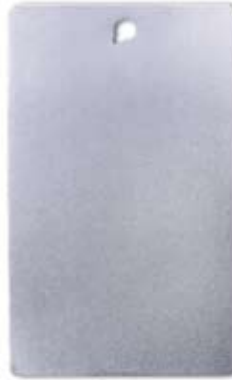
VpCI™ protected mild steel panel
